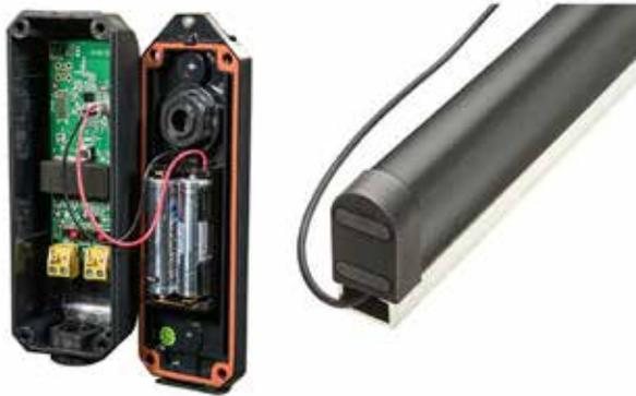
**Wireless Edge:** These are typically only on slide gates, although in some circumstances they may be used on swing gates. If at any time your gate loses connection with the monitored safety edge, the operator will stop functioning. The transmitter box, typically mounted near the edge, needs to be opened and the batteries inside replaced. To ensure regular and consistent operation, these batteries should be replaced annually. Standard AA lithium batteries are recommended.
