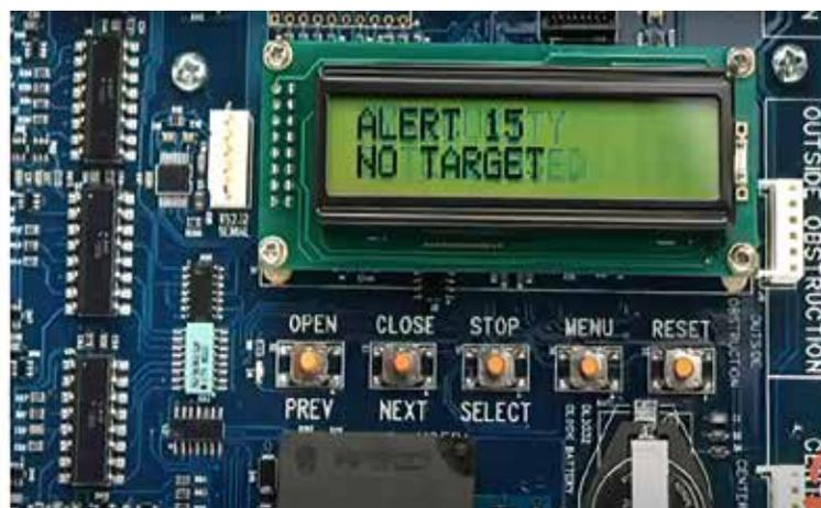
**Check any open commands.** Check that no remotes are being held, that no keypads have an open command, that smart access phone apps are disabled, and nothing is triggering an exit loop or puck.
